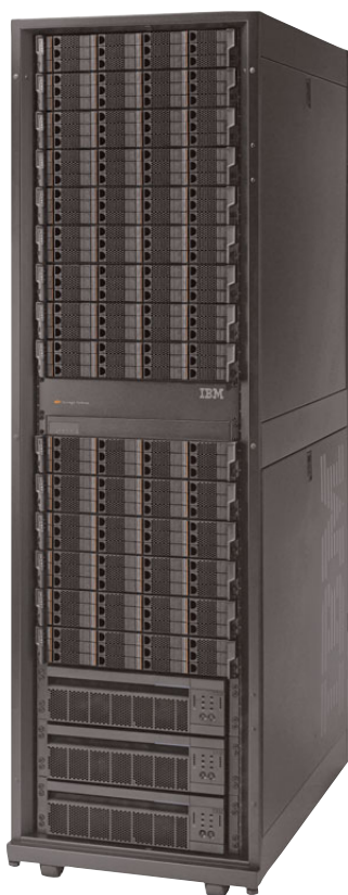
IBM XIV: Single-tier storage based on a scalable grid architecture
